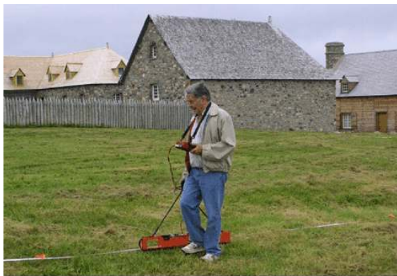
Duncan MacNeill surveying with the EM-38 Conductivity Meter
